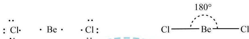
Figure 4. Structure of BeCl<sub>2</sub> molecule from the VSEPR model.
