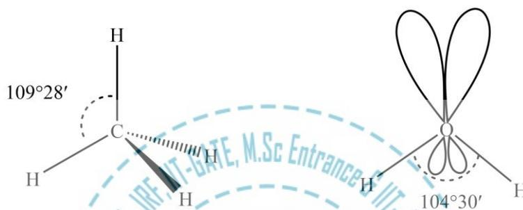
Figure 40. The comparison of the bond angle of methane and water though both have of  $sp^3$  hybridization.
