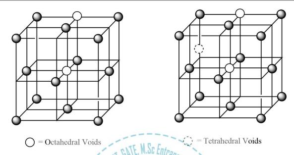
Figure 8. The location of octahedral and tetrahedral sites in cubic close packing or fcc lattices.
