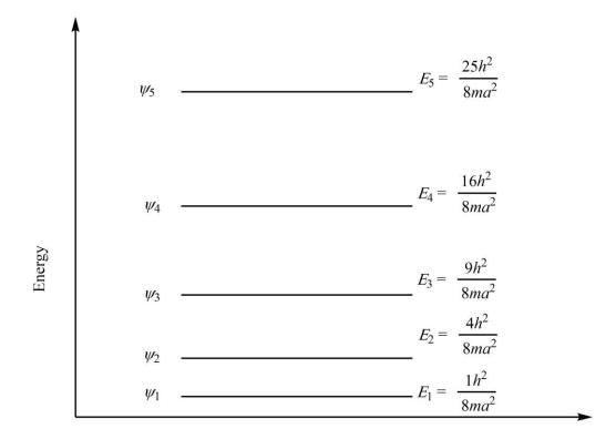
Figure 13. All the energy levels a particle in a one-dimensional box of including the "lowest energy of the particle".
