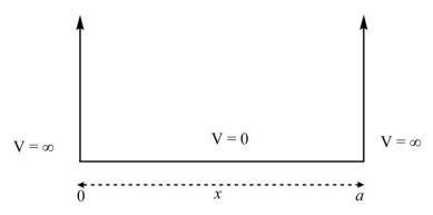
Figure 8. The second representation particle in a one-dimensional box.
