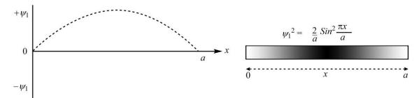
Figure 14. The plot of the wave function (left) and probability for the lowest energy state a particle in one-trapped in dimensional box.
