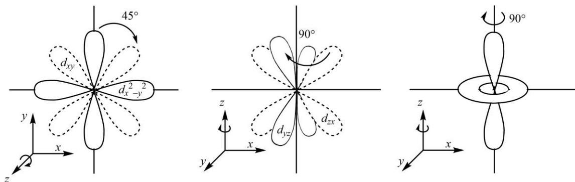
Figure 9. The circulation of electron density in a partially filled  $d$ -subshell about the  $z$ -axis.
