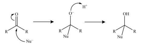
The reaction given above is also called a 1, 2-type nucleophilic addition, and a racemic mixture will be obtained if the alkyl substituents are different.
